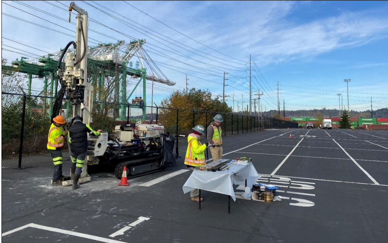
Figure 8. Boring for AB-2 with direct push drill. View northwest.
